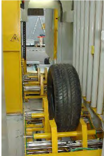
Inlet Conveyor & Transport Carriage
