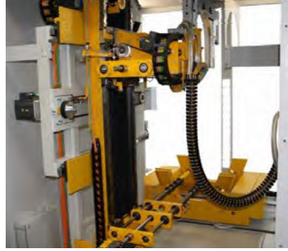
Manipulator - 4 bar spreader in 30 inch bead diameter position (Max.)
