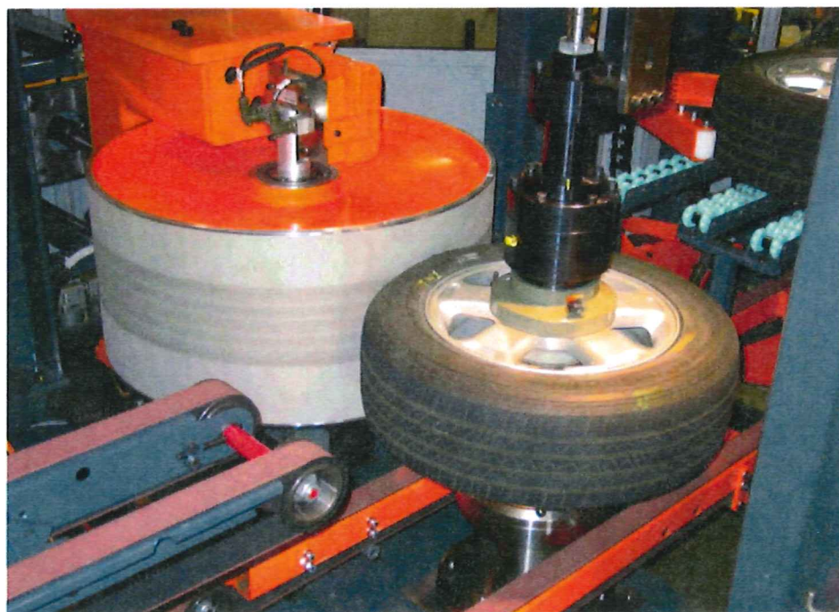
BELOW: The Akron Standard Tire Evaluation Center (ASTEC) measures force variation around the circumference of the tire and wheel assembly when a load is applied that simulates typical vehicle operations
