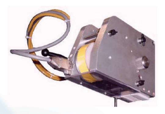
The Akron Standard <sup>®</sup> Hot Stamp Marker is available in kit form and is easily retrofitted to your existing D70, D70 LTX, D90 and FD90 Tire Uniformity Machine. It features an automatically controlled heated pin used to transfer pigment from a tape to the tire sidewall. The Hot Stamp Marker is available in 1, 2, 3 and 4 Pin Models which will allow up to four marking colors at a time.
