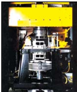
Isolated balance station hard-bearing measurement system.
