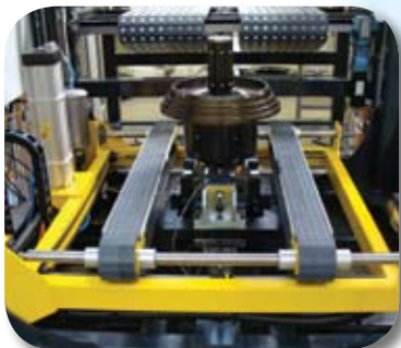
Spindle with measurement devices and transfer conveyor are the heart of the system
