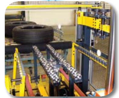
AkroDYNE™ Handler & Luber with tire centering
