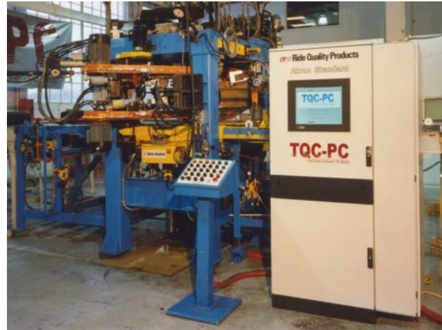
TQC-PC™ controller shown with the Akron Standard Model 70 Series Uniformity Machine
