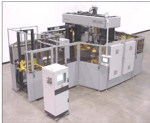
"ERV" Measurement Package is available as an option on the ASTEC® Model "C" Tire Uniformity Machine from Akron Standard™
