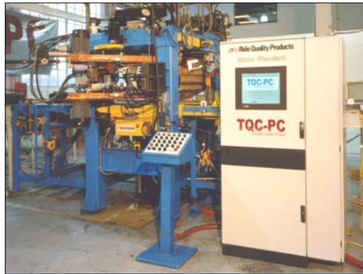
"ERV" Upgrade Kits available for D70 Series Tire Uniformity Machines with Akron Standard™ Tire Quality Controller-PC (TQC-PC™)
